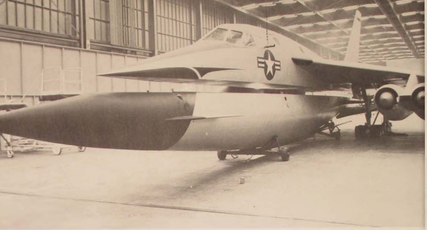
At the Convair Fort Worth plant in 1953, the original B-58 mockup, with bomb and fuel pod lowered, revealed an inherent problem: the nosewheel could not be extended for landing until the pod had been dropped.
